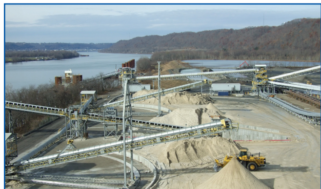
Gypsum at Stuart Station prior to off-site landfilling or commercial reuse in dry wall and other products
